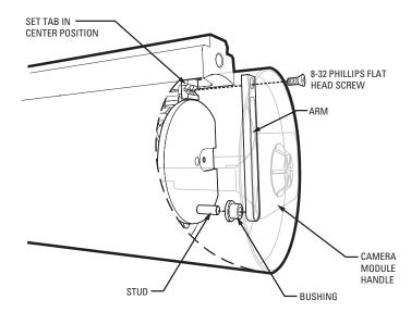
Figure 14. Remove or Install Camera Module
